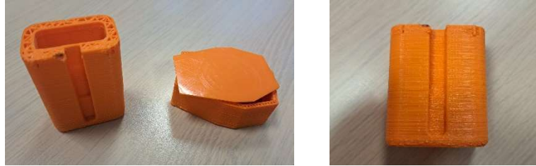
Picture 5&6: Elements of a connector printed by EuraMaterials (test of the material)
