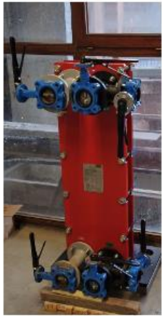
Open Loop Heat Exchanger
