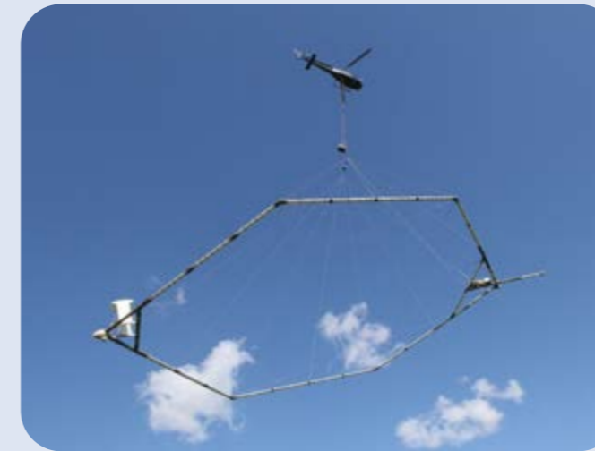
SkyTEM system in the air and an example of the variation of the specific electrical resistivity in the subsurface
