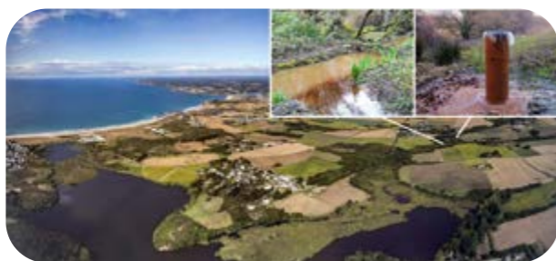
Photo of the coastal Natura2000 classified ecosystem, which is fed by upstream groundwater upflow. On the top right, focus on a wetland upstream the classified ecosystem: artesian well highlighting significant upwelling from deep aquifers, confluence between river (surface water, light brown color) and groundwater-fed river (dark orange color).
