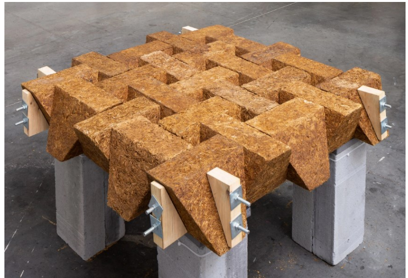
Sugarcrete, a brick made from the sugarcane by-product bagasse (figure 26)
