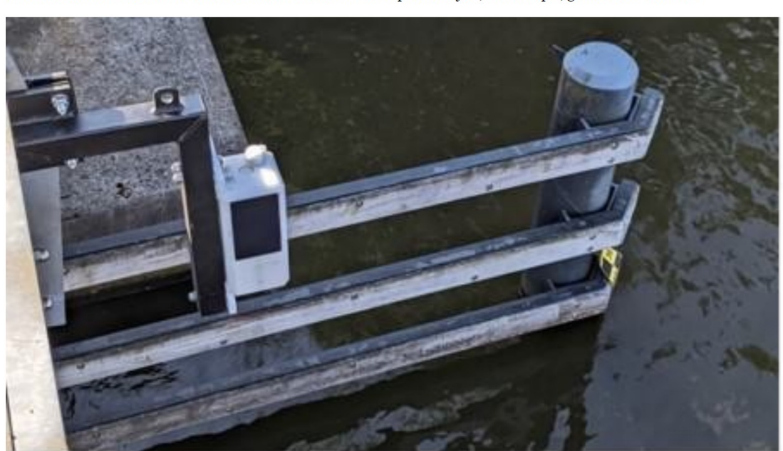
Using a camera and artificial intelligence, the amount of waste that passes under a bridge is counted. © Photo Noria
