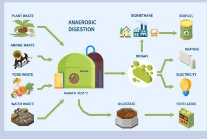
One way to enhance the production of biogas is to mix other organic substances with the feedstock. Sometimes, these additives can make up half of the input volume. The resulting material after digestion, called digestate, can be applied as a biofertilizer.
